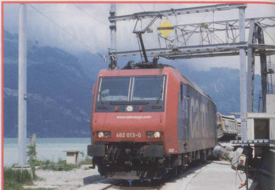
ABOVE: 482013 at the discharge site with Vierwaldstättersee in the background. The yellow diamond with a black stripe above the loco denotes the end of the overhead power supply hence the need to use the front pantograph.
