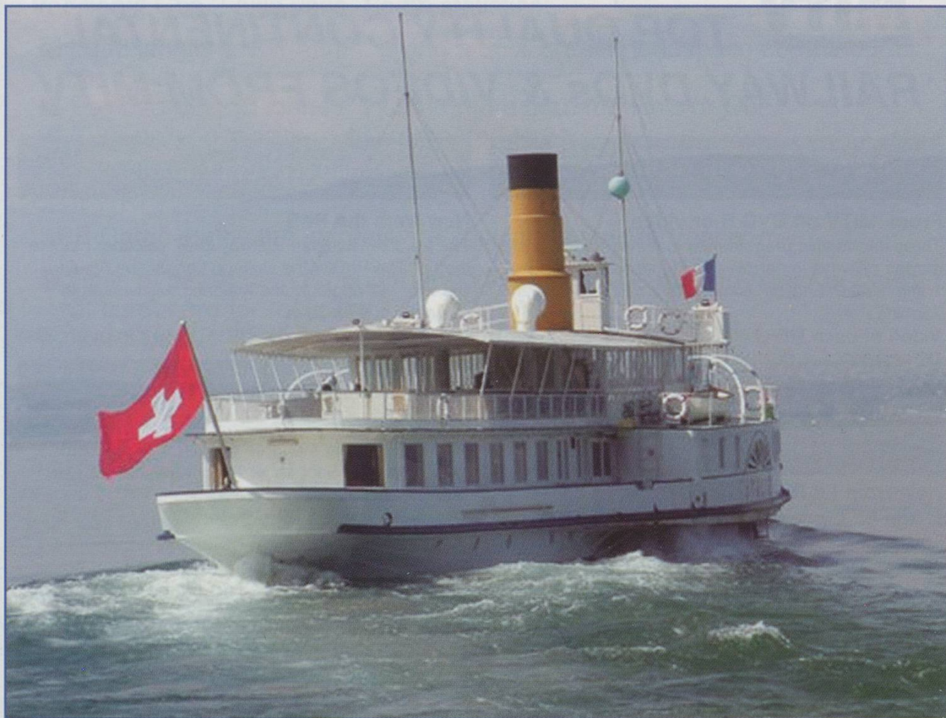
The CGN's ms Italie cruising on Lac Léman. This ship is not a paddle "steamer" as was built, since its paddle wheels are powered by a Sulzer diesel engine. Re-equipping this ship with steam propulsion is now a possibility (April 2005)
