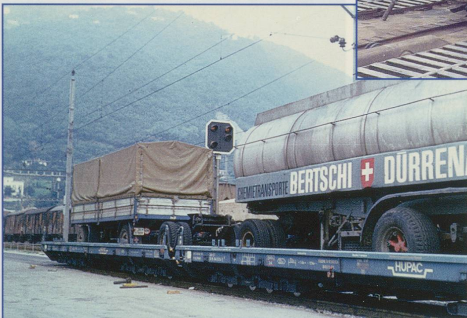
Bertschi drawbar trailer loaded on Wippen wagon
