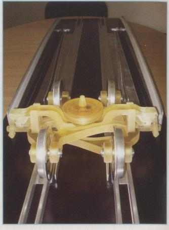
bogie are connected by trapezoidal frames that in their turn are locked together when the bogie is moving. The wheels themselves are on stub axles at either end of the frames.
