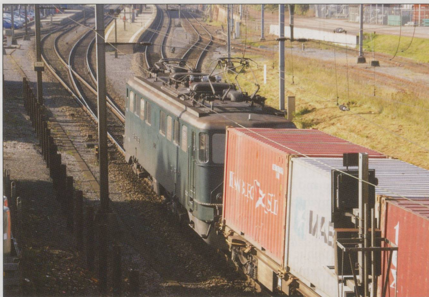
Below: An unusual view of 11473 showing its pantograph gear.
