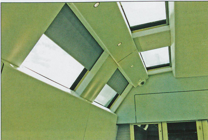
TOP LEFT: General view of Fotoabteil showing seat arrangement and windows in coach Bi57601. The roof blinds are operated by the touch pad to the left of the end door. BOTTOM LEFT: View of panoramic roof windows showing blinds.
