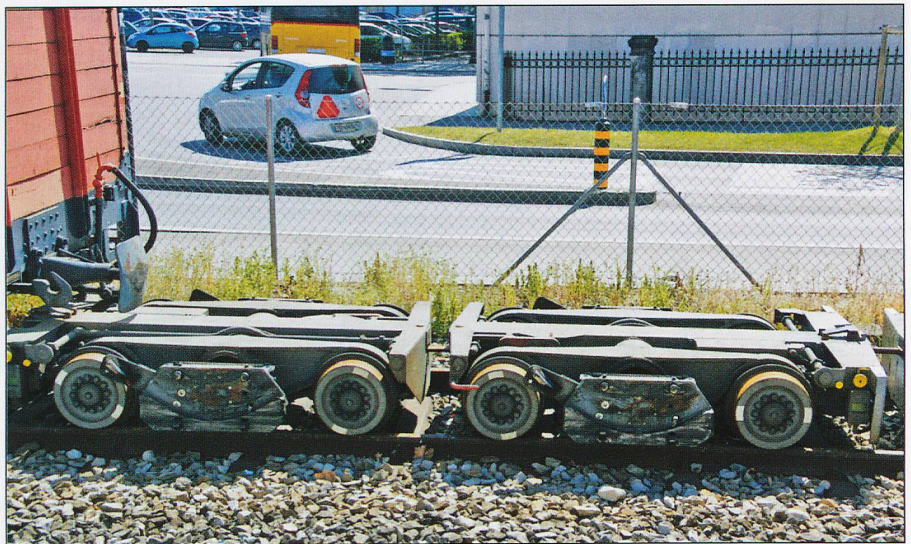
Transporter bogies in the siding at Yverdon.
