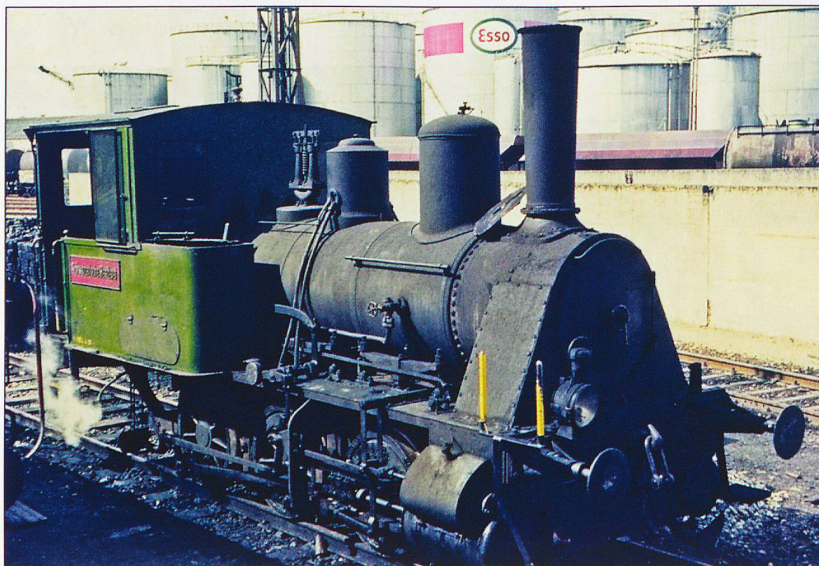
The old T3 0-6-0T shunter of the Schw. Reederei, replaced in the 70s by a Tigerli. (See photo in Part one)
