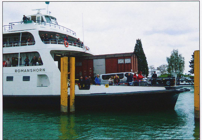
Ferry vessel "Romanshorn" carrying a vintage freight van (formerly Bodensee - Toggenburg K3 no. 1710) that was temporarily placed on a low loader road vehicle for the event. The standard gauge rails that used to be permanently installed on this vessel were removed many years ago.
