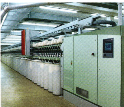
Abb. 5: Rieter Rotor Spinning System
