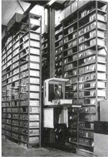
Fig. 14, A typical distribution center, interior view, showing a picker-crane and its driver, in: Joylon Drury / Peter Falconer, Building and Planning for Industrial Storage and Distribution , Oxford: Architectural Press, 2003, p. 171.
