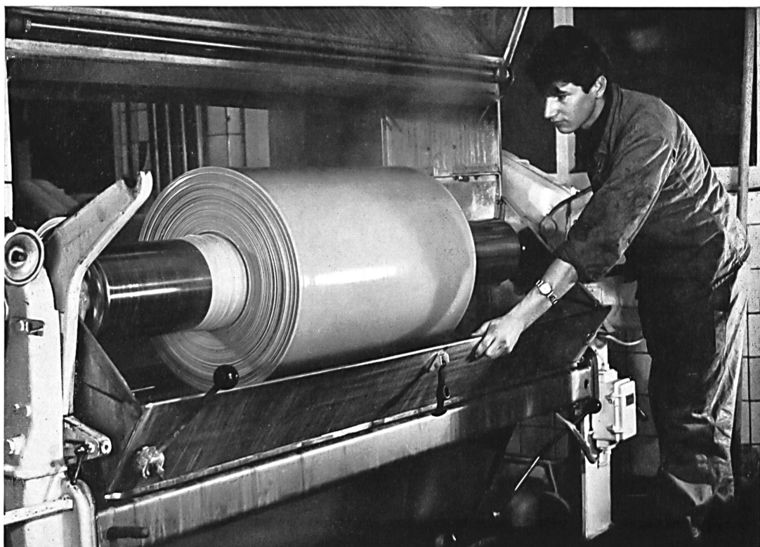
Piece dyeing on an automatic jigger
