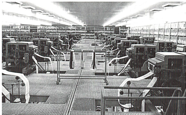
With every loom (bottom of picture), there is a Jacquard machine (top of picture). For the weaving process, it reads the information required for the individual designs from perforated cards and passes it on to the loom.
