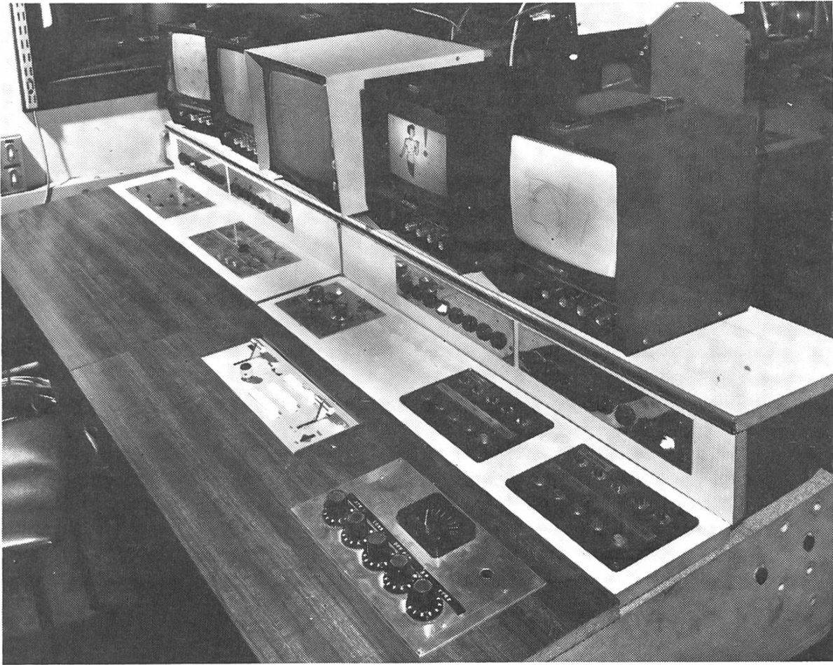
Figure 2: A wide range of visual material can be brought together and mixed into a programme
